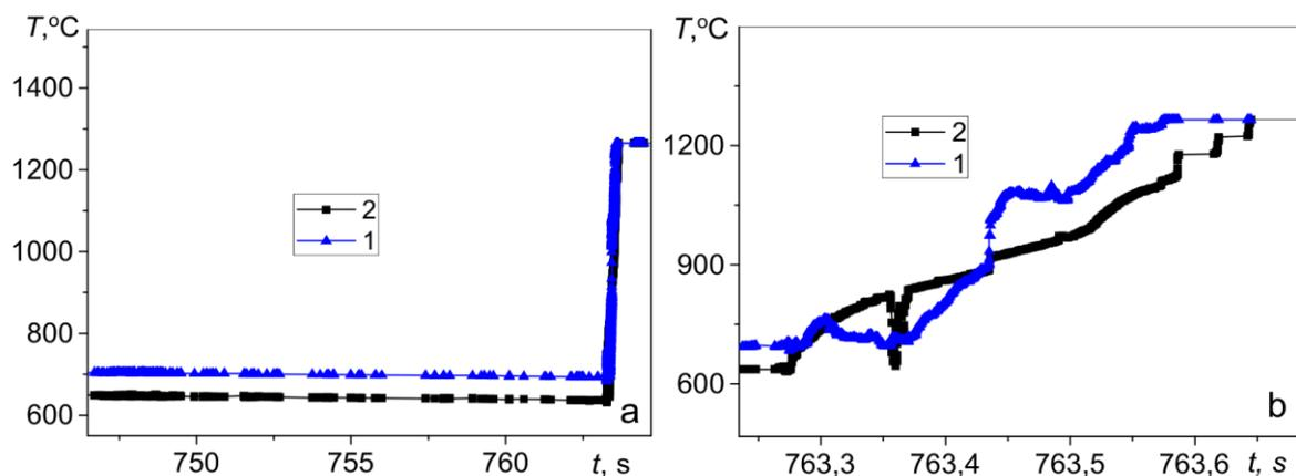
Fig. 3. Thermokinetic of reacting interaction in Nb-Al system: a-general view, b-fragment, indications of thermocouple throughout sample length: 1-2 mm, 2-6 mm.
