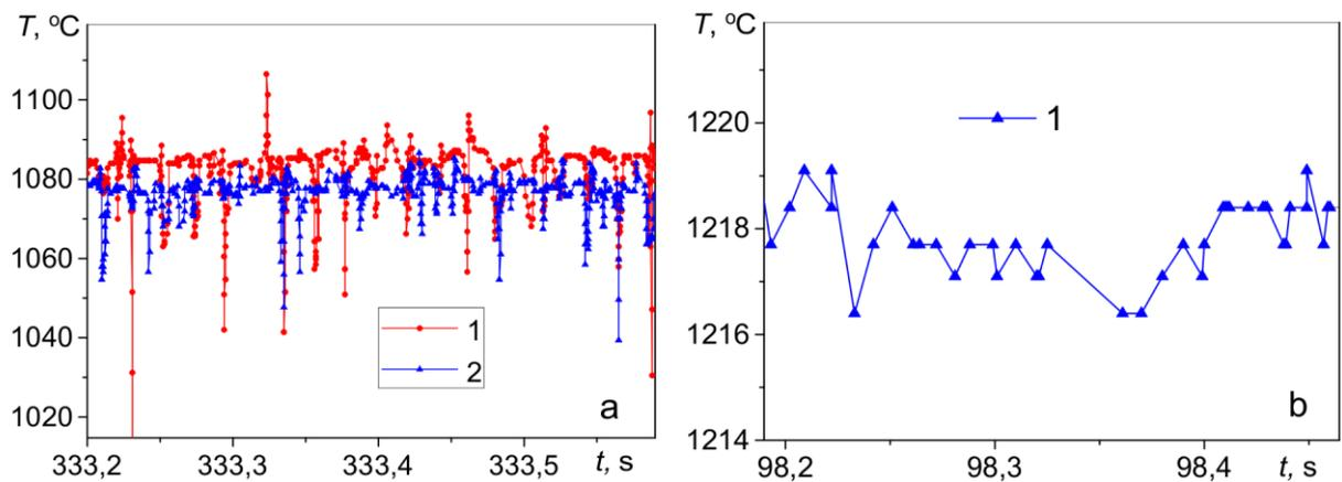
Fig. 8. Thermokinetics of niobium materials oxidation process: a – 37 % Ti, b – 45 % Ti; 1 and 2 - indicated value of thermoelements which are installed on the surface and 2 mm deeper, respectively
