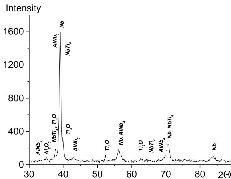
Fig. 6. X-ray diagram of phase composition of alloy on the basis of niobium sintered at 1375 °C during one hour
