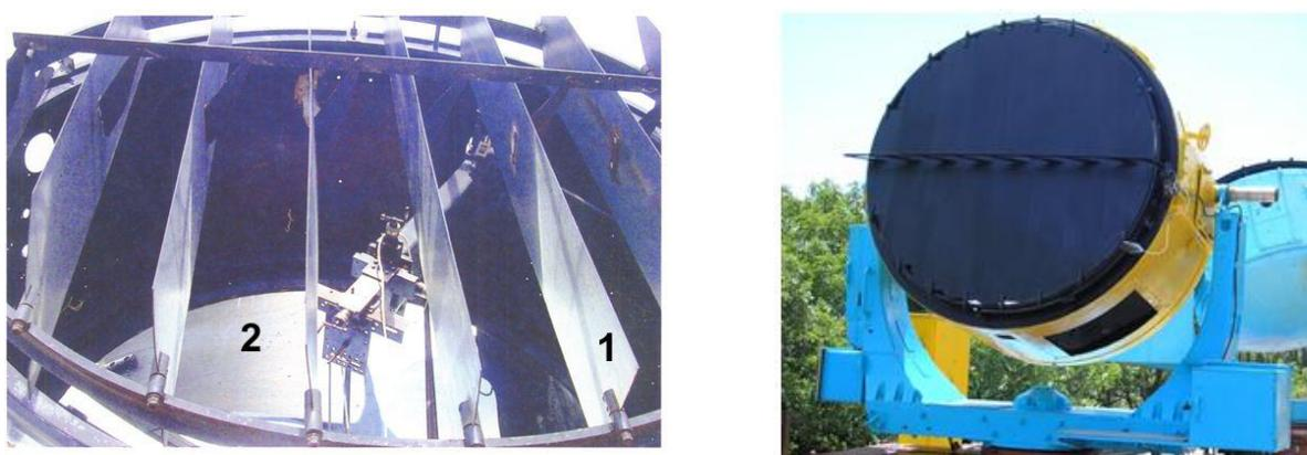
Fig. 1. Solar power plant for studying of thermokinetics of reactionary interaction in obtaining of alloy on the basis of niobium: 1 – sun louver; 2 – paraboloid reflector  $\varnothing$  2 m
