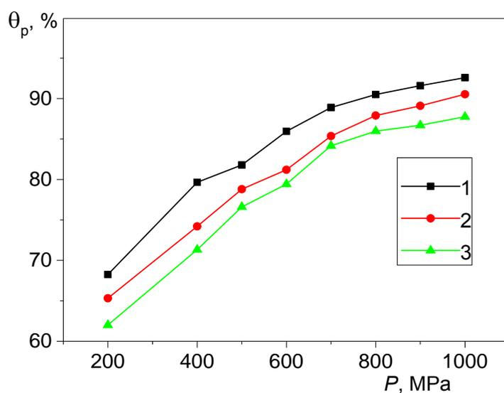
Fig. 2. Dependence of pressing relative density on pressing pressure: 1 – Nb;
