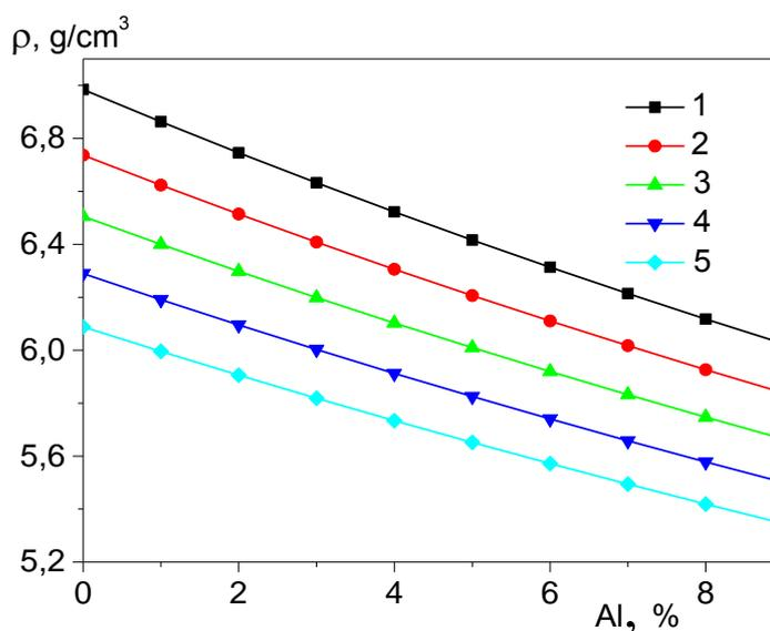
Fig. 4. Dependence of niobium alloys theoretical density on titanium and aluminum containing: 1 – 25% Ti; 2 – 30% Ti; 3 – 35% Ti; 4 – 40% Ti; 5 – 45% Ti.
