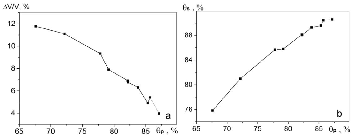
Fig. 5. Dependence of sample(s) shrink-off and its relative density at sintering temperature 1325 °C on density rate of pressing of composition on the basis of niobium with 37 % Ti, which contain aluminum and yttrium oxide. Where  $\Delta V/V$  - samples shrink-off;  $\theta_s$  – density rate of untreated pressings
