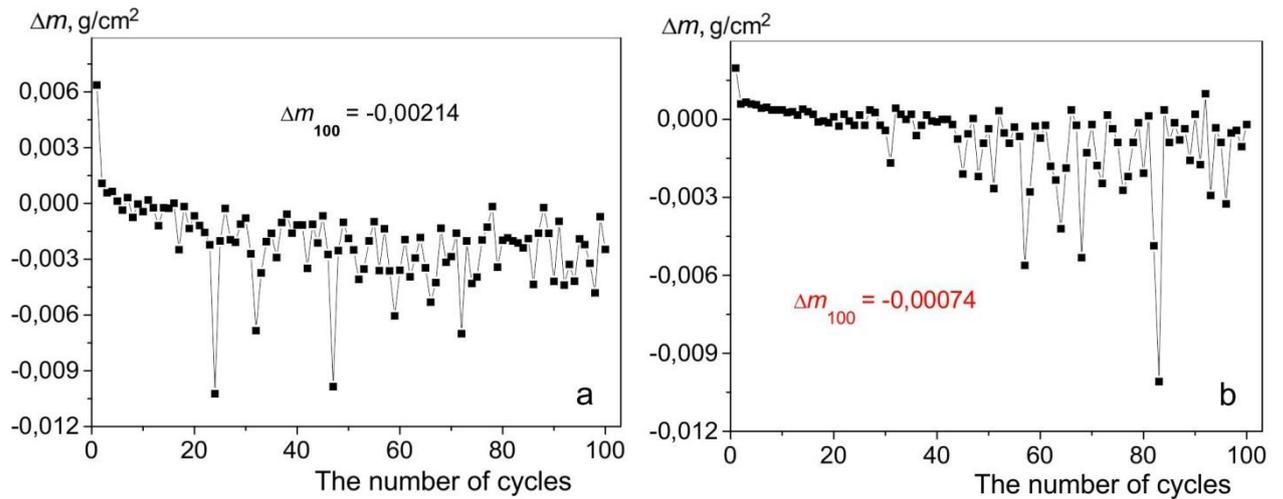
Fig. 7. Cyclic heat resistance of dispersion-strengthening niobium alloy developed with the application of reaction sintering with density  $\rho = 5.788 \text{ g/cm}^3$  (a) and  $\rho = 5.558 \text{ g/cm}^3$  (b) at a temperature  $1200 \text{ }^\circ\text{C}$
